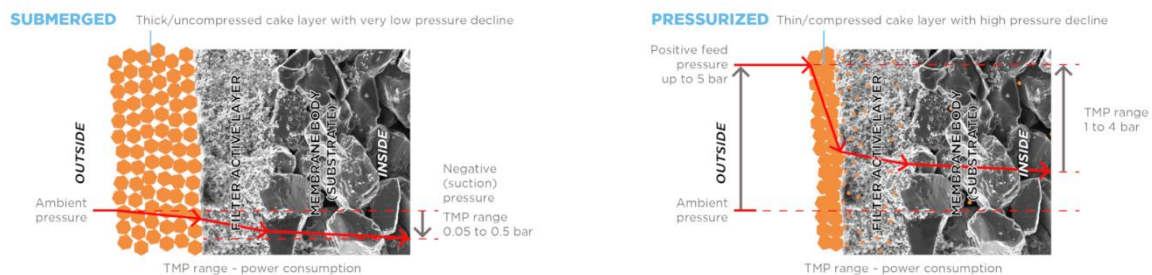
Figure 12: Differences between submerged (out-to-in) and pressurized (in-to-out) Filtration
