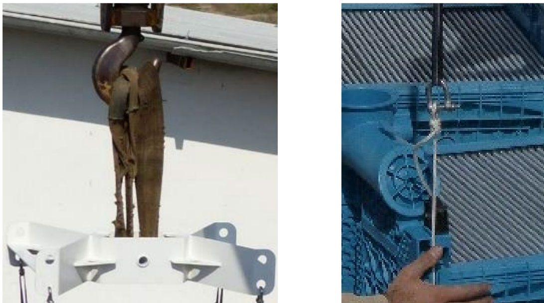
Figure 25: Fixing the tool onto a crane hook (left). Connect coil-loop with rope by shackle.
