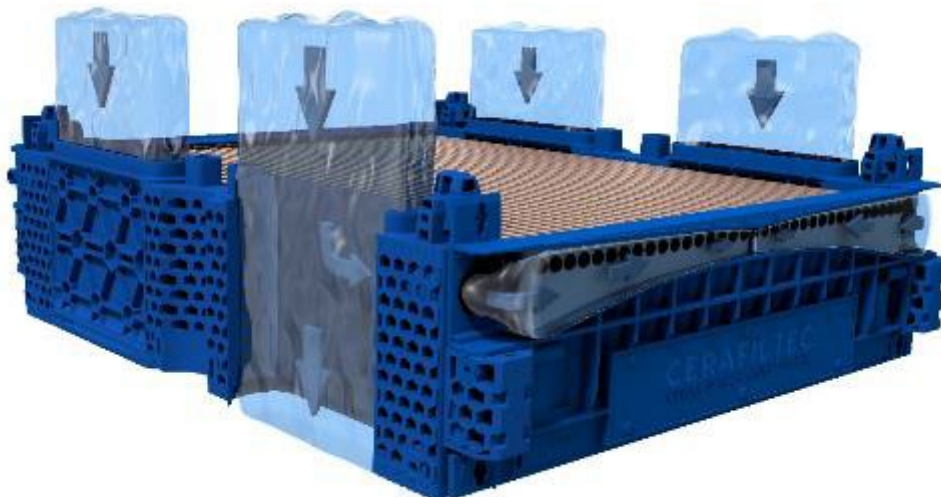
Figure 21: Module principle of backwash process
